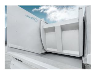
We offer Hardox 450 as an option for extending the useful life of the equipment located in the parts exposed to corrosion.
