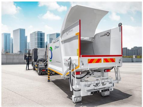
15.It has a bin lifter that allows unloading different types of bins from the top to the body, an openable lid to facilitate manual loading, an ejection plate that allows the waste to be discharged from the body, and a 380V electric motor that runs the entire system.
